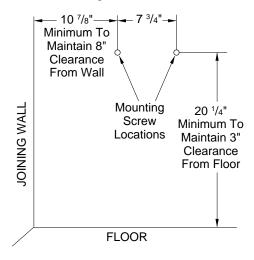
Figure 5 - Mounting Screw Locations
